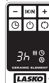
Timer Function in High Heat and Automatic Temperature Control
